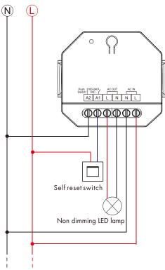
Self reset switch: Short press, turn on the light;
